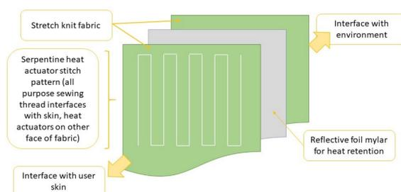
Figure 3: Garment fabric layers schematic [2].
