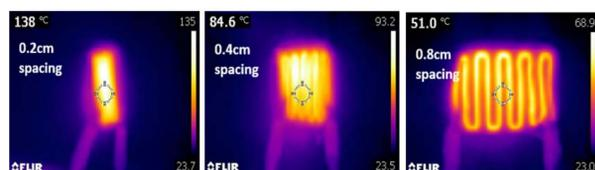
Figure 1: Actuator swatches showing variable trace spacing (top) and corresponding performance (bottom) [1].
