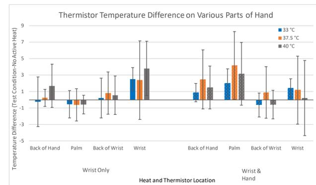
Figure 6: Averaged thermistor temperature difference on various parts of the hand compared to no-heating condition [2].
