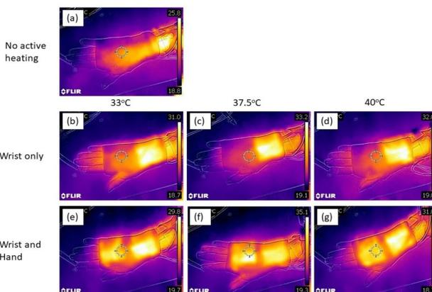
Figure 4: Thermal images for one participant during each test condition. (a) No active heating, (b)-(d) wrist only heat, (e)-(g) wrist and hand heating. Scale values in vertical bar, image right [1].
