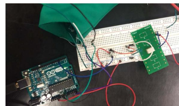
Figure 7: Feedback system using a thermistor input and Arduino Uno® microcontroller to control resistive heating.
