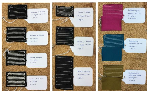
Figure 2: Actuator swatches showing (a) variable trace thickness (b), trace spacing (c), and fabric substrate properties [1].
