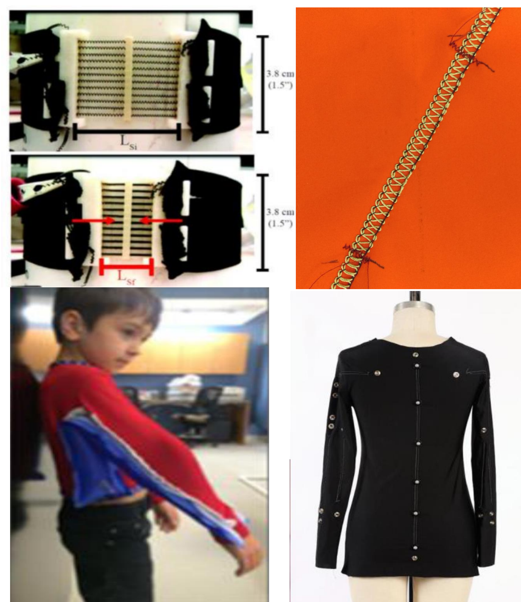
Figure 1: Row 1 (left): SMA Actuators, (right): textile sensor Row 2 (left) pneumatic garment, (right) sensing garment
