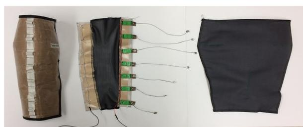
Figure 2. Garment Layers: Base Sleeve (left), Middle Layer (center), Cover (right)
