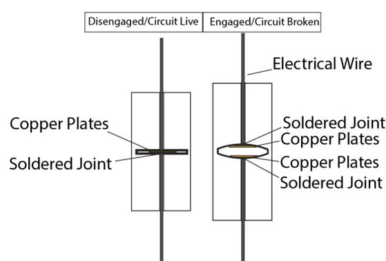
Figure 3. Copper switch diagram
