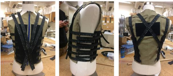
Figure 1: Hook-and- Loop strap test garment (front, side, and back). The graded hook-and-loop straps are anchored on the shoulders and are free to move
