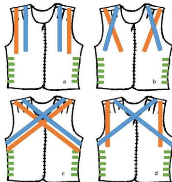
Figure 2: The red straps correspond to the outer shoulder strap, blue straps correspond to the inner shoulder strap, and green straps for torso straps. Test Conditions: (a) Straight, (b) One-side crossed, (c) Two-sides crossed, and (d) Mixed.
